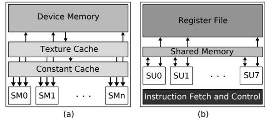
Fig. 2. Organization of the NVIDIA GeForce 8800 series of GPUs
